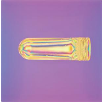
stress patterns of PET bottles measured by PSM-S02 at 0° and 45° white light
