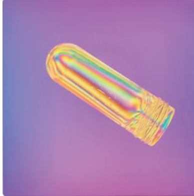
stress patterns of PET bottles measured by PSM-S02 at 0° and 45° white light
