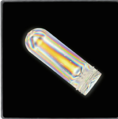
stress patterns of PET bottles measured by PSM-S02 at 0° and 45° white light
